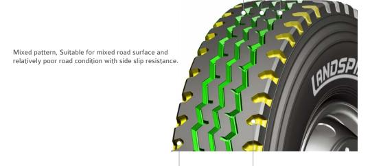
Open Shoulder designs, the block pattern offer excellent drive force and anti-peeling performance on paved and unpaved roads.
